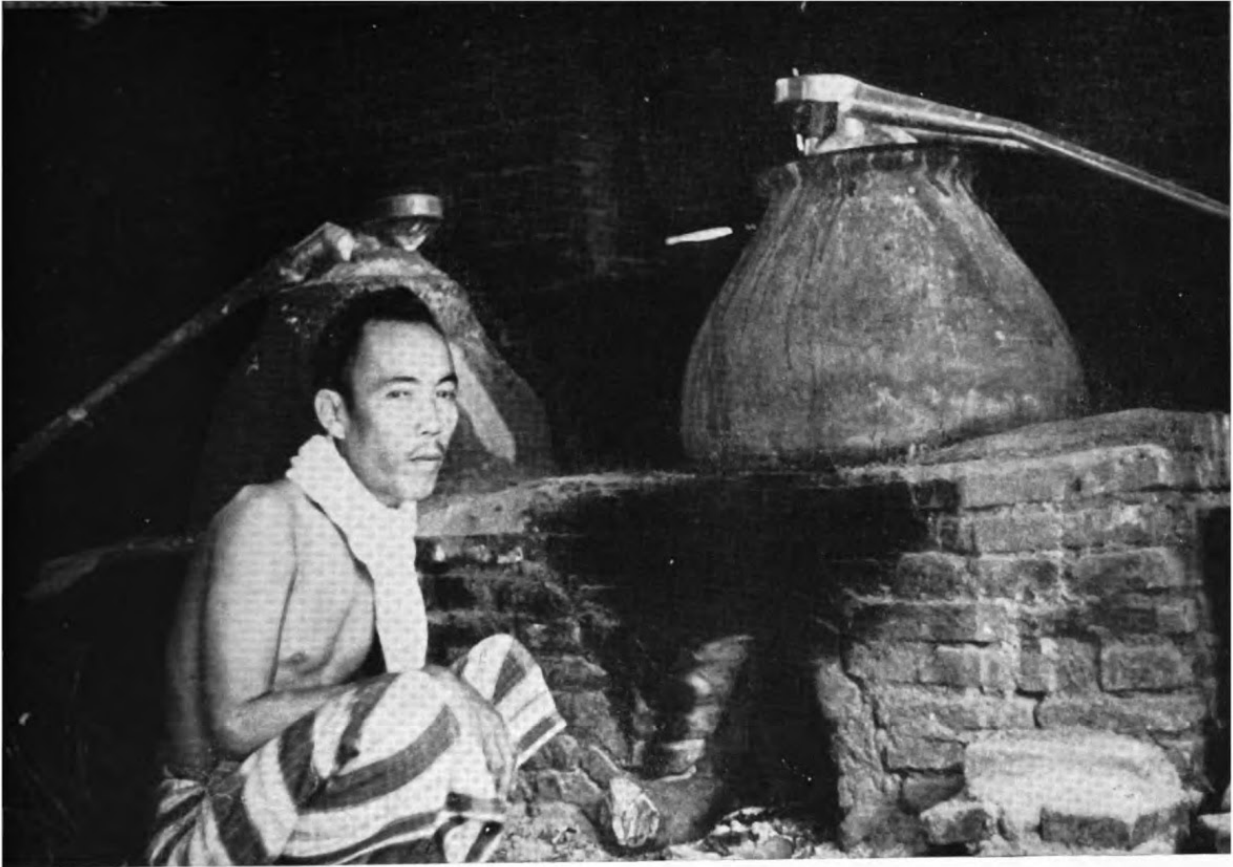
(Top) Production of cananga oil in the Bantam region of Java (Indonesia). Primitive direct fire stills serve for the distillation of the flowers. (Bottom) Cananga oil, Bantam region. View of primitive condensers and oil separators. Photos Fritzsche Brothers, Inc., New York.
